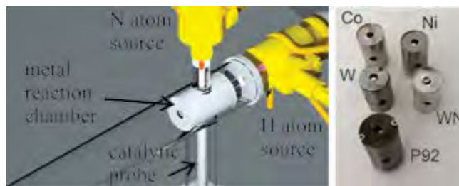
Figure 4: Scheme of the system for determining the coefficient for the conversion of nitrogen atoms into ammonia (left) and reaction sleeves (right) [4].
