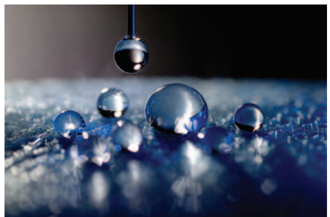
Figure 6: Image shows the dosing of the water drop to the surface of the untreated mask. If the mask is treated the water drop is absorbed.
