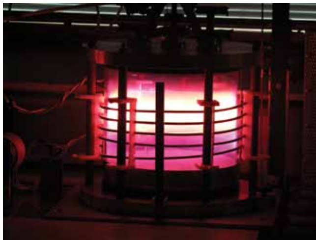
Figure 1: Plasma is created using an inductively coupled RF discharge
