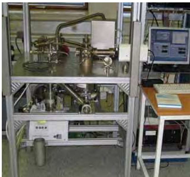
Figure 4: The new, ultra-high-vacuum system for a quantitative analysis of gas mixtures.
